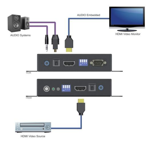
Connect the HDMI Video source at the front panel ports.
