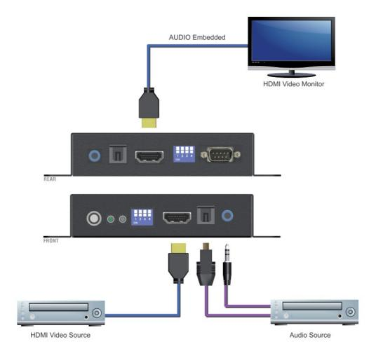
Connect the HDMI Video source and the Audio source at the front panel ports. Select using Mode Switch #1 the type of the Audio source.
